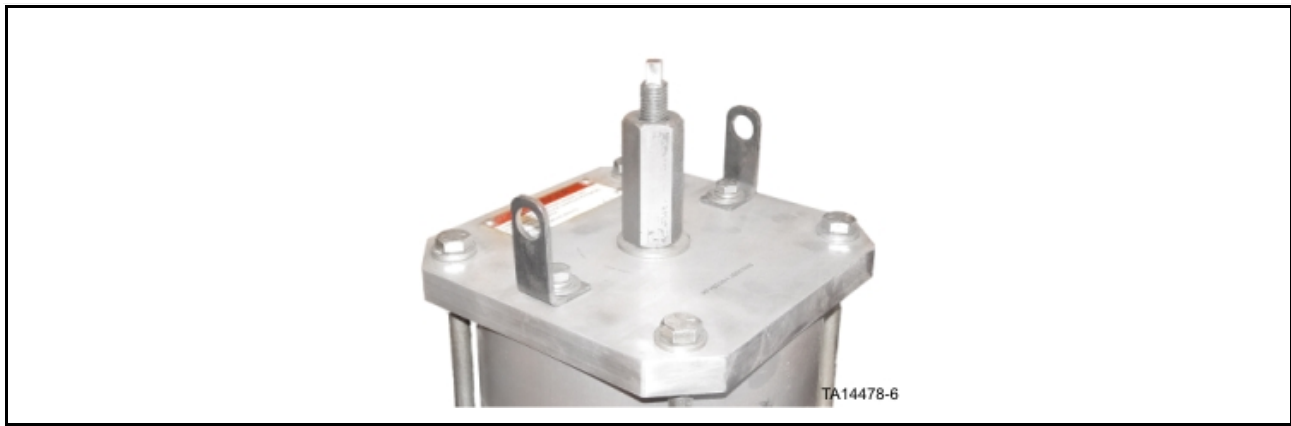
Figure 288. View of jack rod installed in brake cylinder
