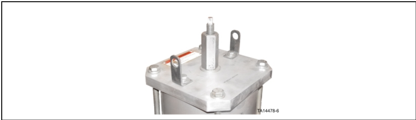
Figure 314. View of jack rod installed in brake cylinder
