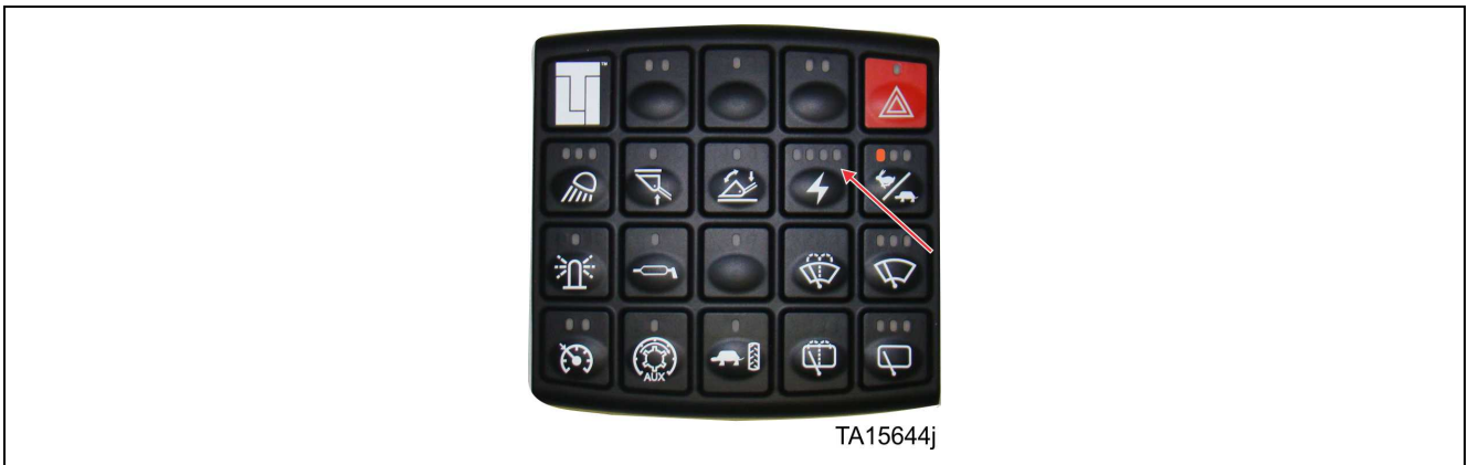
Figure 186. Drive switch power button LED's off
