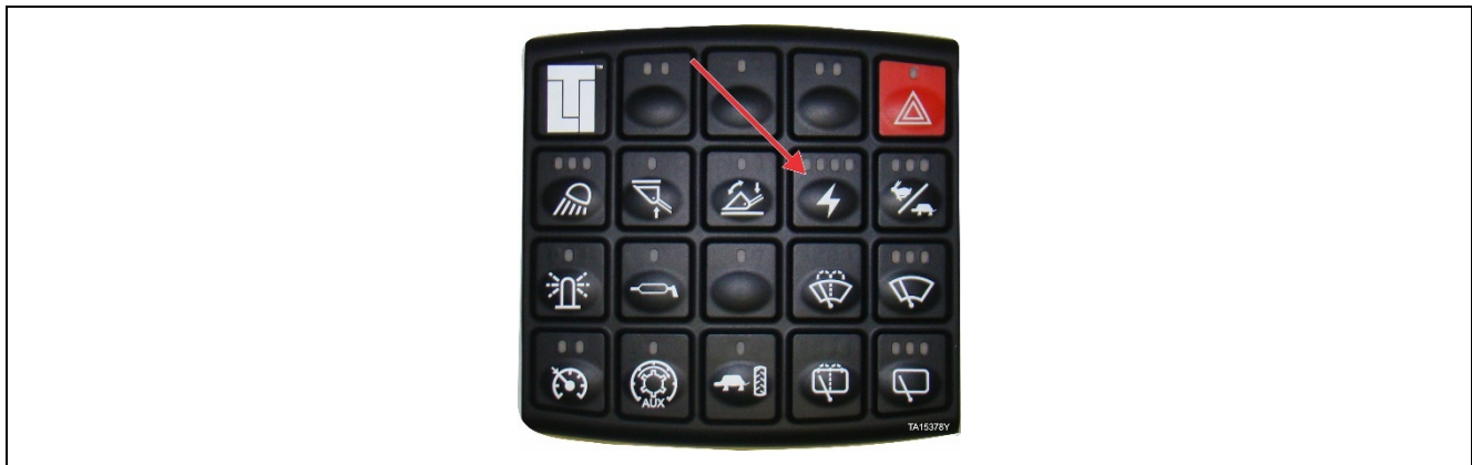
Figure 29. Drive Enable Switch
